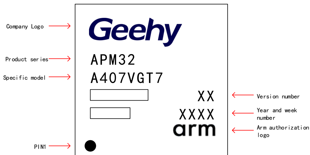
Figure 19 LQFP100 - 100 Pins, 14 x 14mm Package Schematic Diagram
