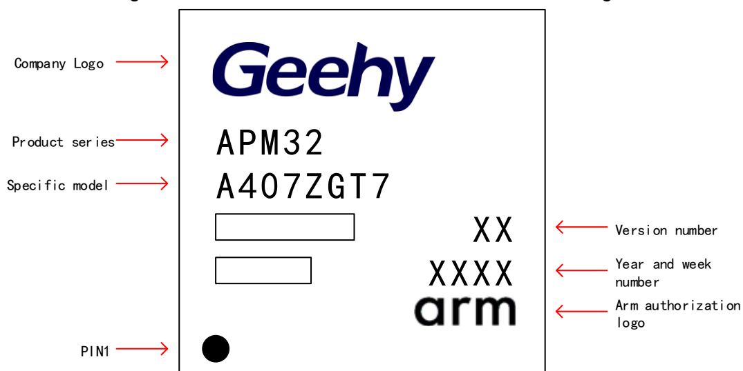
Figure 16 LQFP144 -144 Pins, 20 x20mm Schematic Diagram
